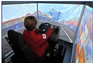
ST-VP is fully containerized real-time distributed HLA Simulator reproducing Port Operations. ST-VP is integrated in a 40' High Cube Container ready to be used on site immediately after arrival.
