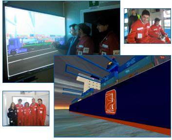
ST-VP includes a full-scope Simulator for Training Crane Operations & Procedures, an Integrated Class Room, the Instructor Debriefing Room, and secondary Interoperable Simulators of Trucks and Other Cranes, Biomedical Module for Ergonomic and Posture Enhancement.
